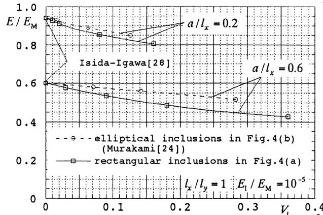
Fig. 6. Relation between  $E / E_M$  and  $V_1$  ( $E_1 / E_M = 10^5$ ).
