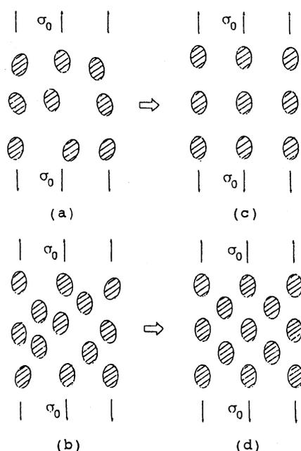
Fig. 1. Periodic arrangement of elliptical inclusions.
