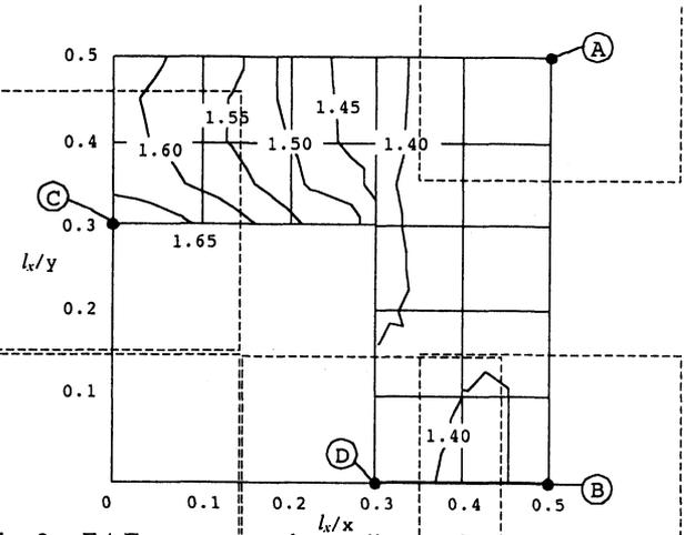
Fig. 9.  $E/E_M$  vs. central coordinate of group B in model (2) ( $b/a=1, l_x/l_y=1, V_1=8ab/(l_x/l_y)=0.18, E_1/E_M=10^5$ ).
