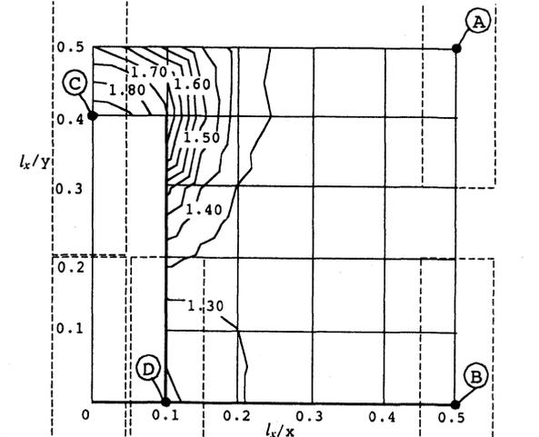
Fig. 10.  $E/E_M$  vs. central coordinate of group B in model (3) ( $b/a=4, l_x/l_y=1, V_1=8ab/(l_x/l_y)=0.08, E_1/E_M=10^5$ ).
