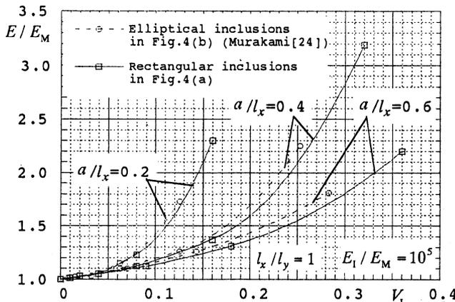
Fig. 5. Relation between  $E / E_M$  and  $V_1$  ( $E_1 / E_M = 10^5$ ).
