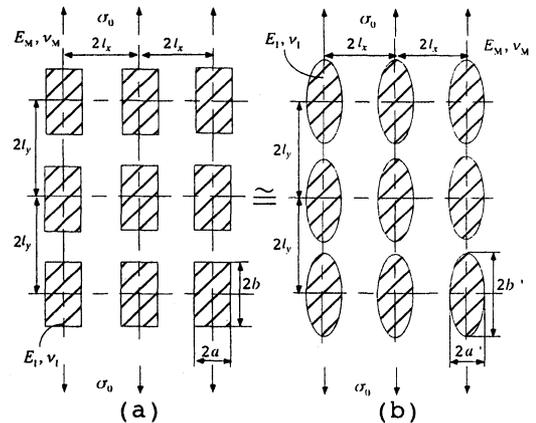
Fig. 4. Elastic modulus is almost equal when (1)  $a/l_x = a'/l_x$  and (2)  $ab/(l_x l_y) = \pi a' b' / (4l_x l_y)$ .
