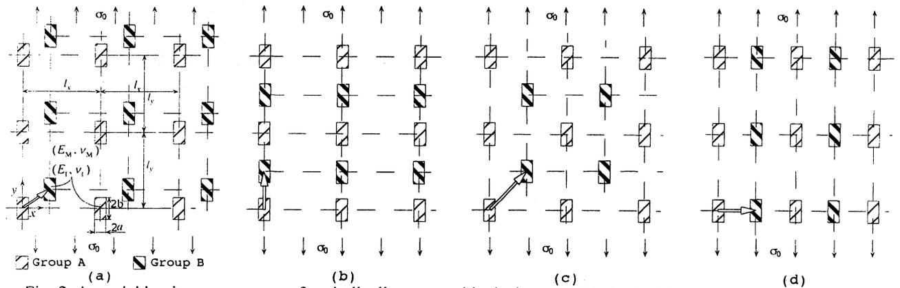
Fig. 2. A model having two groups of periodically arranged inclusions: (a) Model in this study (b) Square array 1 (c) Hexagonal array 2 (d) Square array 2.
