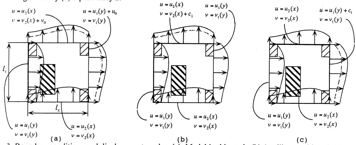
Fig. 3. Boundary conditions and displacement modes: (a) Model in this study (b) Auxiliary problem (1) (c) Auxiliary problem (2).
