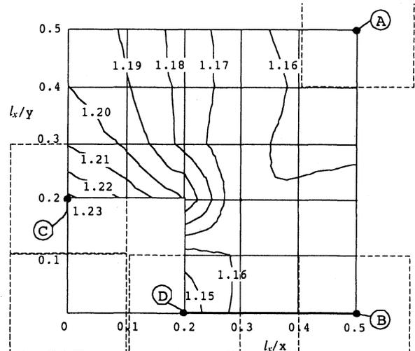
Fig. 8.  $E/E_M$  vs. central coordinate of group B in model (1) ( $b/a=1, l_x/l_y=1, V_1=8ab/(l_x/l_y)=0.08, E_1/E_M=10^5$ ).
