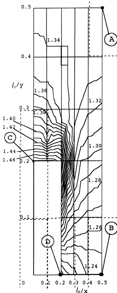
Fig. 11.  $E/E_M$  vs. central coordinate of group B in model (4) ( $b/a=4$ ,  $l_x/l_y=4$ ,  $V_I=8ab/(l_x l_y)=0.08$ ,  $E_I/E_M=10^5$ ).
