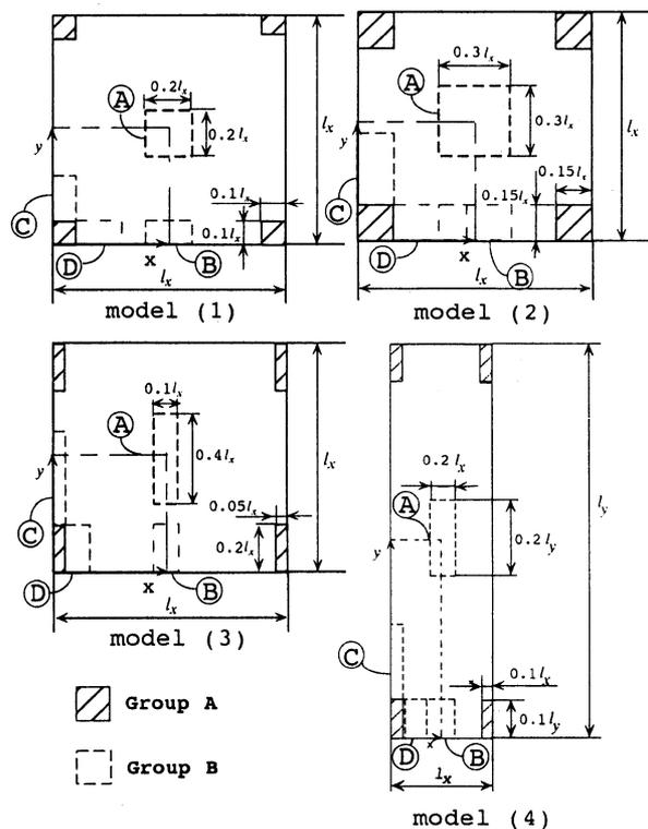
Fig. 7. Models of two groups of periodically arranged inclusions.
