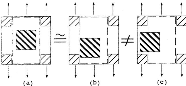
Fig. 12. Effective Young's modulus is almost equal in (a) and (b), but not equal in (c).
